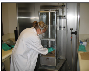
Figure 2. Anesthetized Bombus impatiens being placed in a Potter spray tower for treatment.
