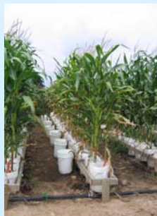
Fig. 1b. Pails covered with plastic bags to control water supply.
